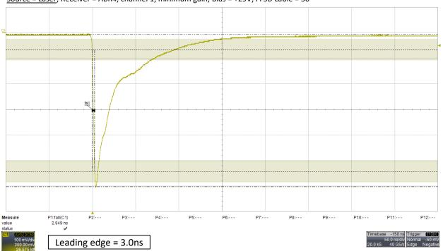
Source = Laser; Receiver = ABR4, channel 1, minimum gain; Bias = +29V; FFSD cable = 36"
