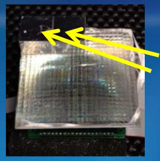
Two samples of 1.5mm pitch LYSO arrays placed in the corner of the tapered Agile light guide placed over the B array.
