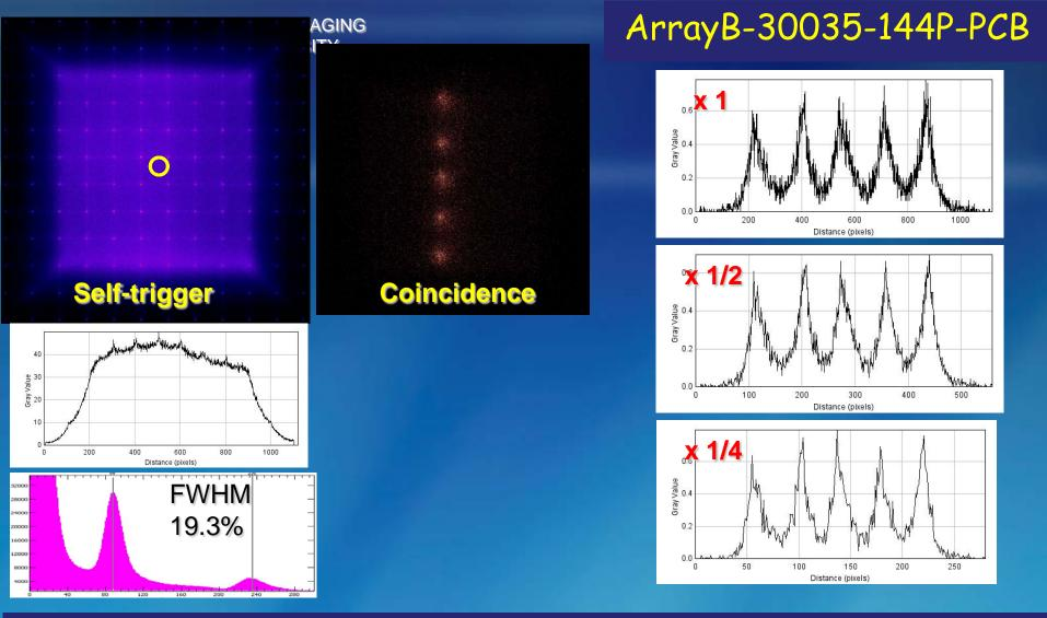
Measurements with the 21mm thick LYSO module. The module was placed directly on the B array. Five Na22 sources placed at a 6,5mm pitch. Quadratic algorithm (R. Pani). Truncation factor (-)0.025. Bias voltage 31.7V. 145 ns wide ADC gate. The coincident profile plot was also compressed 2 and 4 times for better visualization. Estimated spatial resolution ~ 2mm FWHM. Some artifacts seen in the flood image at left primarily due to LYSO radioactive background.
