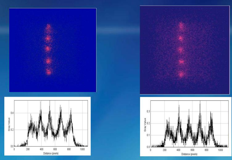
Measurements with 5 sources placed at 6.5mm pitch with the 21mm thick LYSO module. Light guides were placed between the scintillator and the B array. Left: fiberoptic with 1mm square elements, from Agile. Right: thin fiberoptic. In both cases amplitude dropped by about 15-20% compared to the direct coupling. Quadratic algorithm. Truncation factor (-)0.025. Bias voltage 31.7V. 145 ns wide ADC gate. No improvement in resolution.
