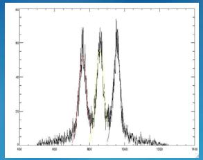
Spatial resolution measurements with electronically collimated 511 keV beams. Left: five <1mm Na22 sources placed at 6.5mm pitch. Right: three 0.5mm capillaries with F18 solution placed at 5mm spacing. The best results show uniform spatial response with about 1.8-2.0mm FWHM. As experimentally confirmed, this limit in resolution is not due to geometry or source size.
