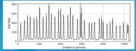
with Measurements the 1.57mm pitch pixellated 10mm thick and 57mm x 57mm LYSO array with the tapered light guide (matching the SiPM array size) from Agile. No spreader window. Bias voltage 29.5 V. 145 ns gate to ADC, truncation factor 0.05.
