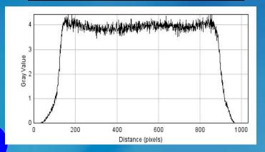
Combination of white top, optimized spreader window, quadratic COG algorithm and energy cut eliminating lower amplitudes originating in the edge regions, produces uniform response across the active surface with energy resolution in the range 12-14 % @511 keV.
