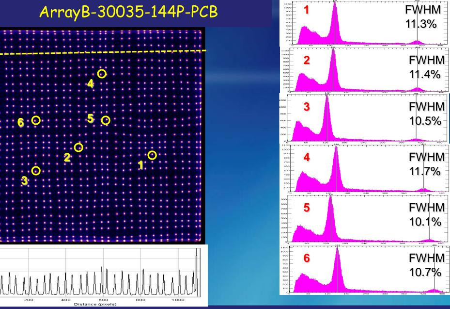
For comparison, measurements with the 1.57mm pixel size 10mm thick and 57x57 mm transversal size LYSO array. 2.1mm thick spreader window was used between LYSO array and SiPM array to produce more uniform spatial response. Bias voltage 28.4V.
