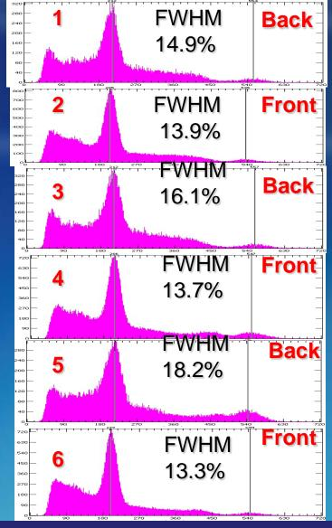
Measurements with two stacked/shifted 1.5mm pitch pixellated 10mm thick LYSO arrays and 2.3mm spreader window. Bias voltage 30.1 V. 145 ns signal integration gate in ADC, truncation factor 0.05. Energies corrected for thresholding effect due to the diode circuitry.
