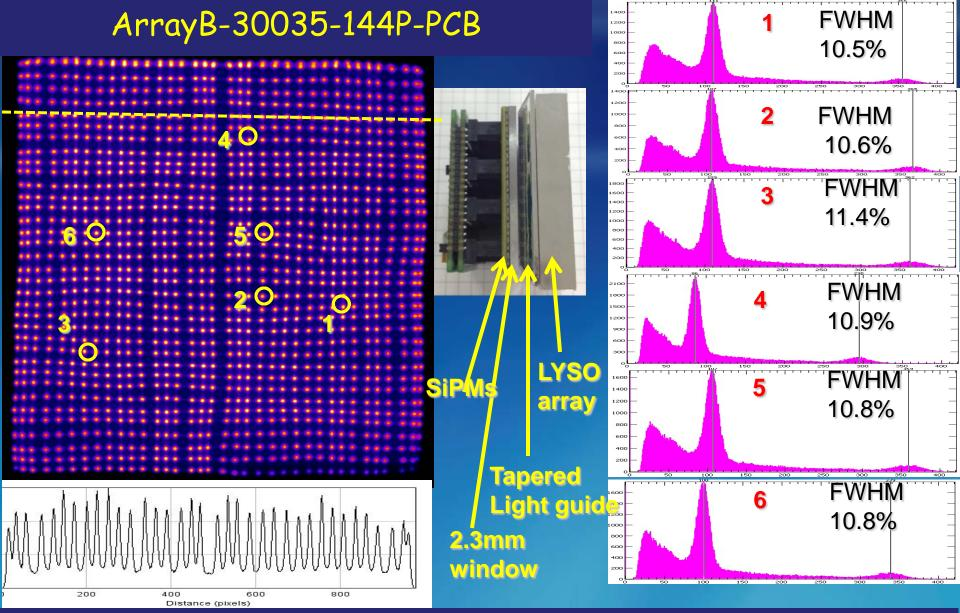
Measurements with the 1.57mm pixellated 10mm thick and 57mmx 57mm on a side LYSO array and the tapered light guide (matching the SiPM array size) from Agile. An additional 2.3mm spreader window is used to produce more uniform spatial response. Bias voltage 28.7 V. 145 ns gate to ADC, truncation factor 0.05. Energies corrected for energy cut due to diode circuitry.
