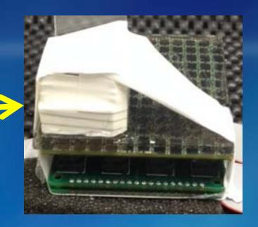
Measurements with two stacked/shifted 1.5mm pitch pixellated 10mm thick LYSO arrays and 2.3mm spreader window.
