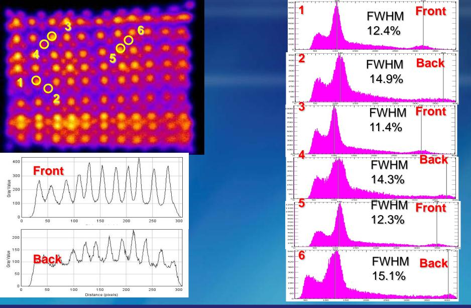
Measurements with two stacked/shifted 1.5mm pitch pixellated 10mm thick LYSO arrays with a tapered light guide and a 1.6mm spreader window placed between scintillator and tapered light guide. Bias voltage 30.1 V. 145 ns signal integration gate in ADC, truncation factor 0.075. Energies corrected for thresholding effect due to the diode circuitry.
