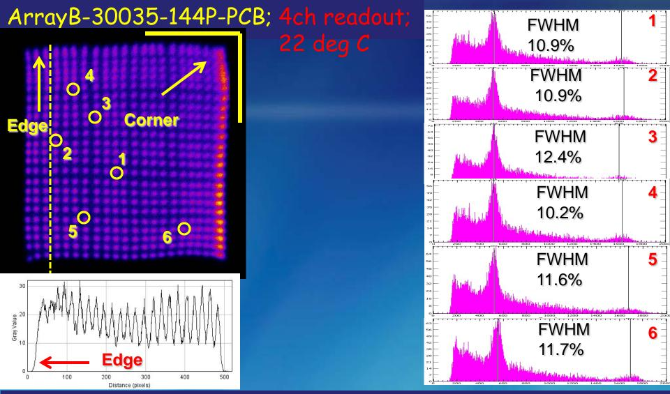
1.0 mm pixel size 10 cm thick Agile/Proteus LYSO array coupled to the SiPM array via 2.75mm spreader window. LYSO array was placed in the corner of the SiPM array. Bias voltage 28.4 V. COG truncation factor 0.075. Examples of a profile and six energy spectra for 1.0mm LYSO pixels. The peak positions were corrected for zero energy shift (thresholding) effect produced by the diode circuitry. Image blurring effects at the edges observed due to higher noise level (higher temperature).
