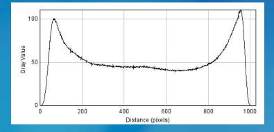
For comparison, measurements with the WVU 1cm thick by 5 cm  $\times$  5 cm LYSO crystal from Proteus with all sides polished, and standard straight black-painted side walls and white top shows serious response non-linearity with heavy edge effects.
