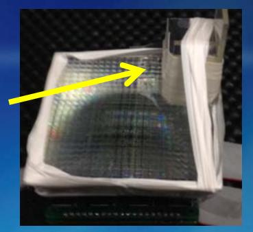
Measurements with two stacked/shifted 1.5mm pitch pixellated 10mm thick LYSO arrays and tapered light guide with several spreader windows.
