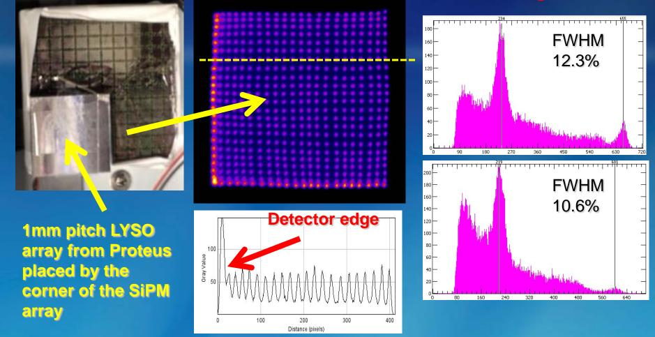
Measurements with a 1mm pitch 10mm thick LYSO array (24x24 pixels). 2.75mm thick UV acrylic light spreader window placed between the array and the SiPM module. Linear algorithm. Truncation factor 0.05. Bias voltage 29.5V. 145 ns wide ADC gate. Two examples of single LYSO pixel energy spectra. Energy peaks corrected for the thresholding effect due to diode charge division circuitry. Slight saturation seen in the 1274 keV peak (from Na22 course)
