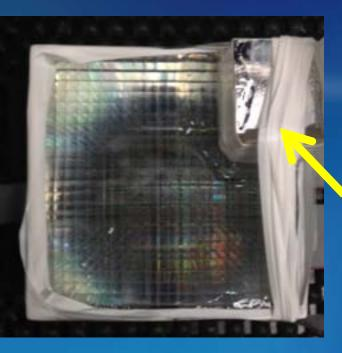
Sample of stacked/shifted 1.5mm pitch LYSO arrays placed in the corner of the tapered Agile light guide placed over the B array.
