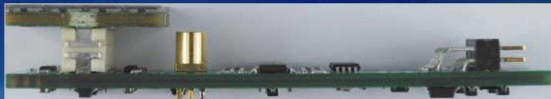
The SiPM arrays is mounted on a stand-off connector, as shown in this side-view picture.
