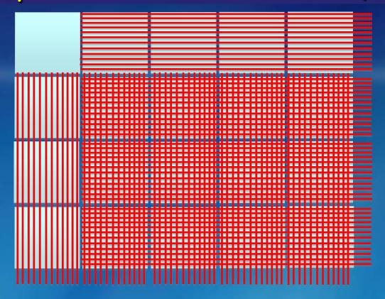
In this schematic example of the 4x5 array of SiPM modules forming  $\sim 25x20cm$  detector panel, in the 144 SiPM modules the initial number of 480 R&C readout channels is reduced to 48 rows and 60 columns =108 MR&C channels. For Array 8 the MR&C channel number will be 36+40 = 72 for  $\sim$  the same size panel.
