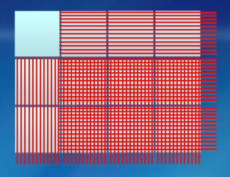
In this schematic example of the 3x4 array of SiPM modules forming ~ 20x15cm detector panel, the corresponding row and column outputs from individual modules are connected together (multiplexed - passively or actively) to form common row and column readout lines for the whole detector panel. For the 144 SiPM modules the initial number of 288 R&C readout channels is reduced to 36 rows and 48 columns = 84 MR&C channels. For Array 8 the channel number will be 56 for the same size panel.
