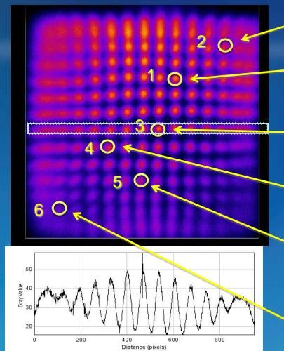
NaI(Tl) array of  $3\times3\times6$  mm pixels coupled to SiPM module through 6.5mm glass window. Bias  $\sim +30$ V. 21.5 C. 600ns signal integration gate. F factor 0.15. Co-57 energy spectra from six selected pixels, FWHM energy resolutions @122 keV and relative peak amplitudes.
