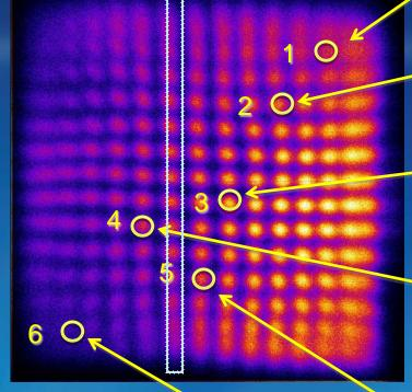
NaI(Tl) array of  $3\times3\times6$  mm pixels coupled to SiPM module through 6.5mm glass window. Bias  $\sim +28.8$ V. 21.5 C. 600ns signal integration gate. F factor 0.125. Co-57 energy spectra from six selected pixels, FWHM energy resolutions @122 keV and relative peak amplitudes.
