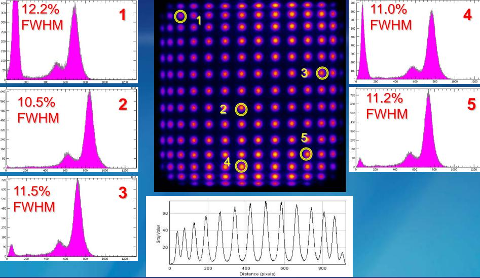
Bias: -1000 V. 520 ns ADC integration gate. Row and column (R&C) readout. Truncation factor 0.075. Energy spectra and FWHM energy resolution values @ 122 keV for five selected Na(Tl) pixels are shown.
