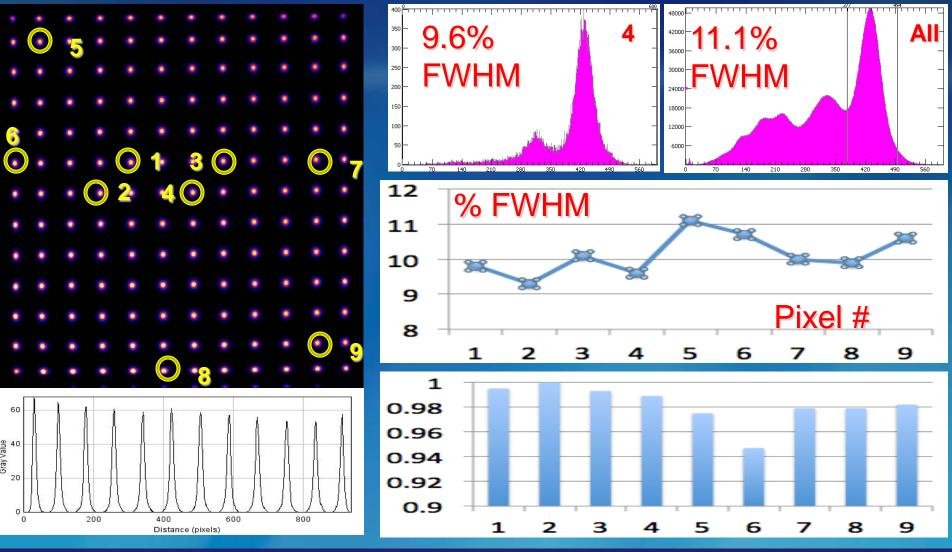
Bias: -900 V. 520 ns ADC integration gate. Row and column (R&D) readout. Truncation factor 0.025. Nine selected NaI(Tl) pixels: FWHM values and relative amplitudes @122 keV are shown. Single pixel energy spectrum (from pixel 4), and from the whole module are also given.
