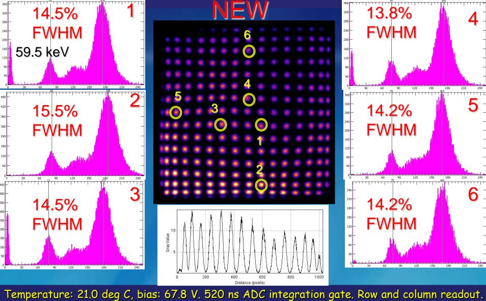
Truncation factor 0.025. Six NaI(Tl) pixels across the surface of the MPPC detector module were selected to measure the FWHM energy resolution of the 122 keV photopeaks. The 59.5 keV photopeaks from low intensity Am241 was used to provide energy scale calibration.
