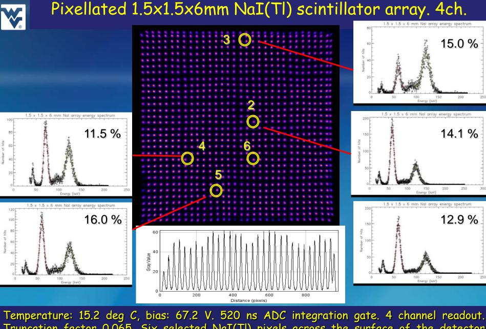
Truncation factor 0.065. Six selected NaI(Tl) pixels across the surface of the detector module. Shown five energy spectra obtained for a combination of Co-57 and Am-241 sources to calibrate zero energy channel. Values of FWHM in % are given for the 122 keV photopeaks.
