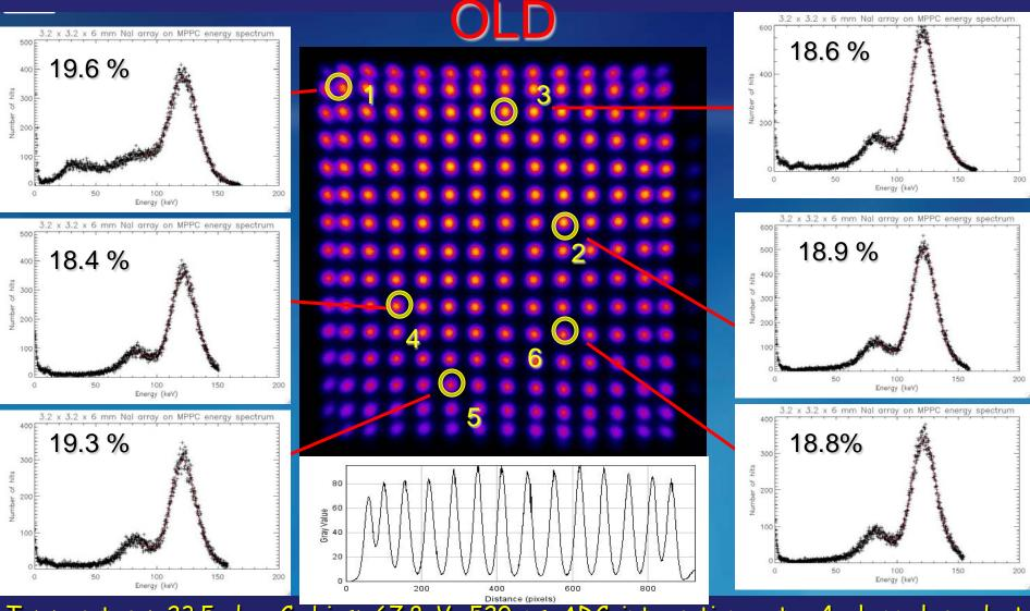
Temperature: 23.5 deg C, bias: 67.8 V. 520 ns ADC integration gate. 4 channel readout. Truncation factor 0.065. Six NaI(Tl) pixels across the surface of the detector module were selected to measure the FWHM energy resolution of their 122 keV photopeaks. The values were NOT corrected for the zero channel energy shift due to diode-based circuitry.
