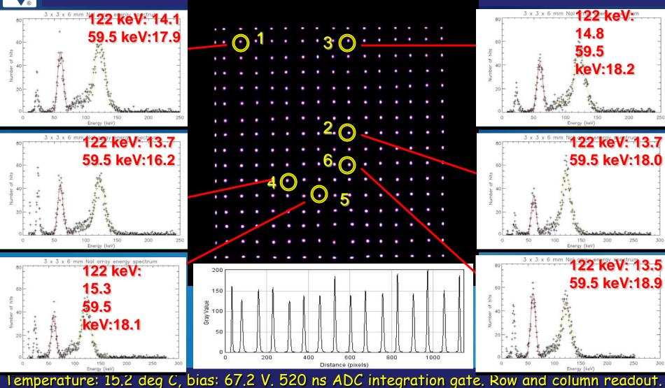
Truncation factor 0.065. Six selected NaI(Tl) pixels across the surface of the detector module. Shown six energy spectra obtained for a combination of Co-57 and Am-241 sources to calibrate zero energy channel. Values of FWHM in % are given for 59.5 keV and 122 keV photopeaks.
