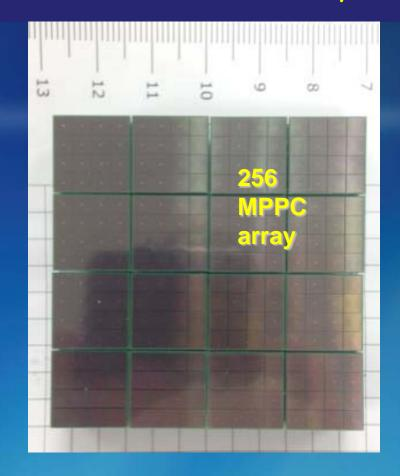
256 element MPPC array was tested with several 1,5 and 3mm NaI(Tl) arrays from Saint Gobain, coupled directly without an additional window to the MPPC array. Visilox V-788 optical coupling compound was applied between the MPPC array and the NaI(Tl) arrays.
