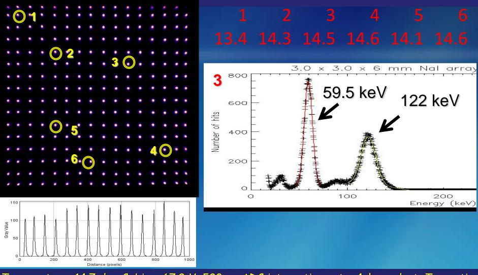
Temperature: 14.7 deg C, bias: 67.2 V. 520 ns ADC integration gate. 4ch readout. Truncation factor 0.05. Six selected NaI(Tl) pixels across the surface of the detector module. Shown an example of energy spectrum obtained for a combination of Co-57 and Am-241 sources to calibrate zero energy channel. Table at top right gives values of FWHM in % for the 122 keV photopeaks.
