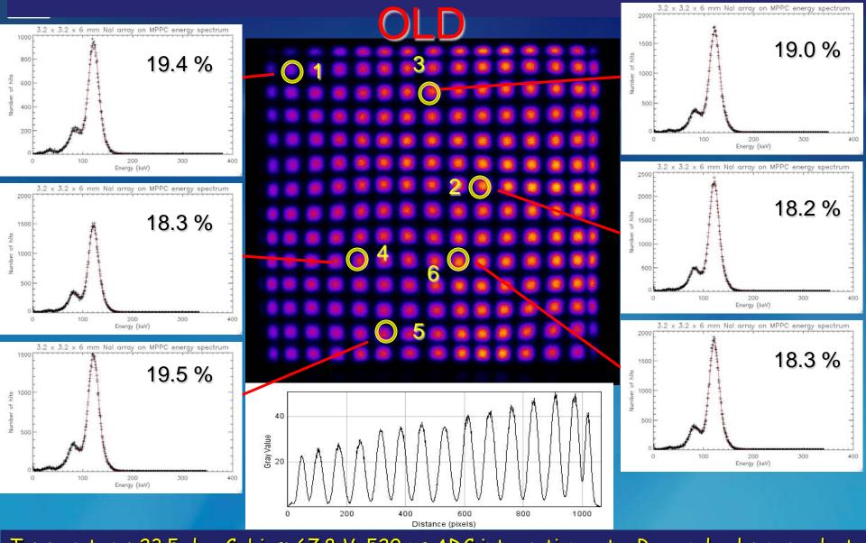
Temperature: 23.5 deg C, bias: 67.8 V. 520 ns ADC integration gate. Row and column readout. Truncation factor 0.065. Six NaI(Tl) pixels across the surface of the detector module were selected to measure the FWHM energy resolution of their 122 keV photopeaks.
