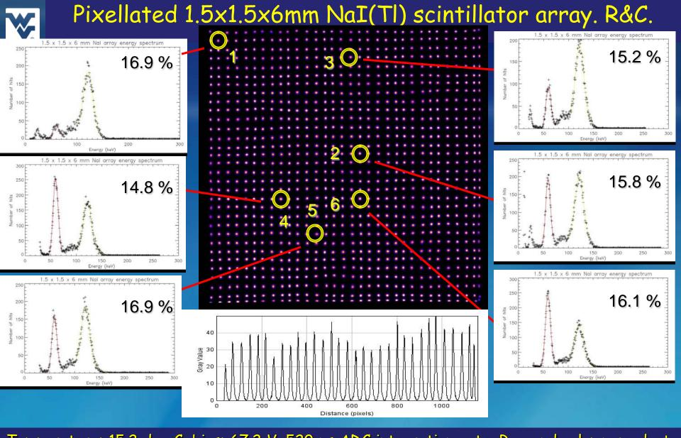
Temperature: 15.2 deg C, bias: 67.2 V. 520 ns ADC integration gate. Row and column readout. Truncation factor 0.065. Six selected LYSO pixels across the surface of the detector module. Shown six energy spectra obtained for a combination of Co-57 and Am-241 sources to calibrate zero energy channel. Values of FWHM in % are given for the 122 keV photopeaks.
