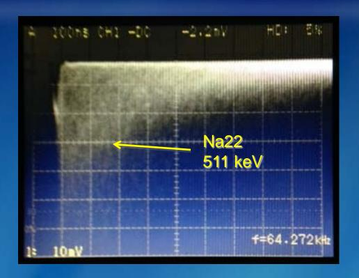
The output from the combined MPPC sum signal of the 4ch AiT charge division circuitry is shown here on the scope screen. Na22 source.
