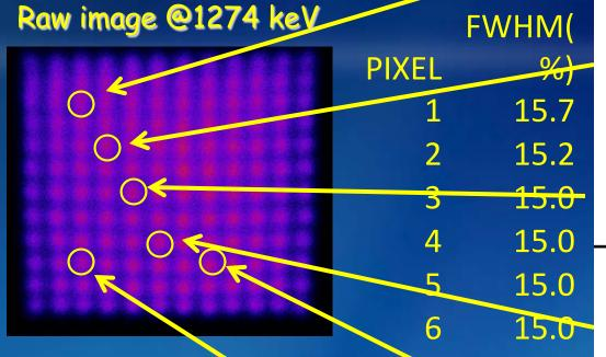
To establish operational limit, post-amplifier system was implemented with spectroscopic EG&G/Ortec amplifiers. I microsec shaping was applied to pulses from the original Jefferson Lab charge division H8500 circuitry, before digitizing the four signals in the standard DAQ module with integrating ADCs. Energy spectra for six selected 2x2x15mm BGO pixels were recorded using 1500 nsec ADC gate. Energy resolution FWHM Q511 keV for each of these pixels is indicated in the table above.
