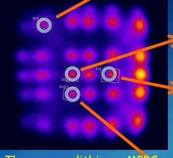
The monolithic MPPC module equipped with 16ch readout from AiT Instruments. FWHM values at 511 keV peak. Room temperature.
