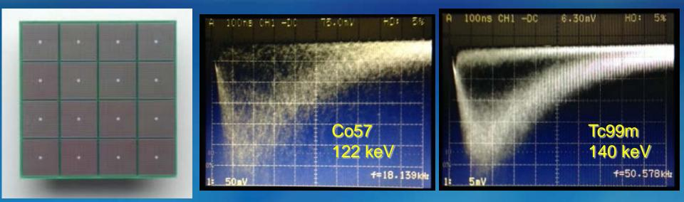
Study of the single-gamma operation using 1.5mm and 3mm NaI(Tl) arrays and AiT 4ch readout:
